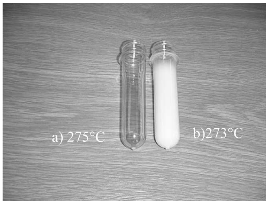
Figure 8. Resin C is a homopolyester that crystallises fast and its haze-clearance temperature is high; (a) transparent preform molded at 274–276°C; (b) lowering the injection temperature to 272–274°C makes the preform completely opaque.
